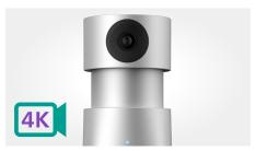
The camera shows speakers in remarkable clear 4k video with accurate color rendition. The 1/2.8 inch CMOS sensor ensures bright, clear video and sharpness even in low light settings.
